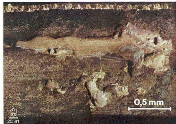
Figure 15. Erosive corrosion point in the free tube length (CuZn28Sn).
