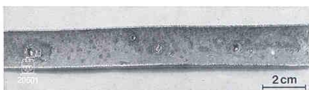
Figure 6. Sporadic pitting in a condenser tube ( \text{CuZn20Al} ) after six years of operation.
