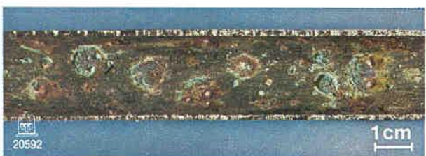
Figure 5. Abundant pitting in an auxiliary cooler tube ( \text{CuNi10Fe} ) at the end of the first few operating months.
