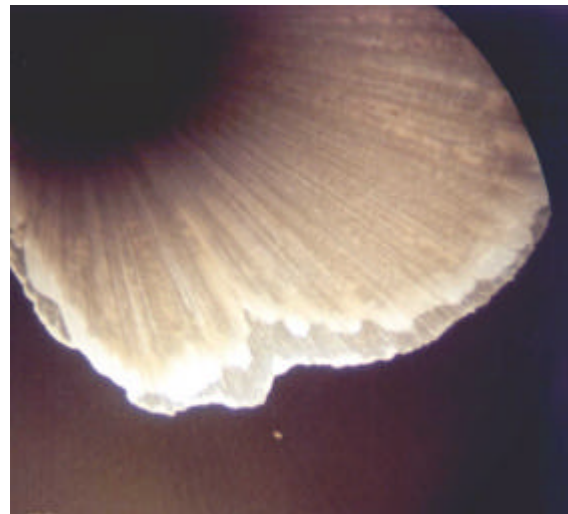
hard calcium carbonate scale
